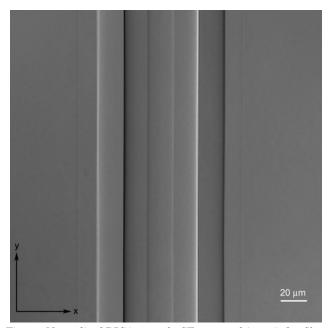
Fig. 1. Normalized DIC image of a CF2-082 multistep-index fiber covering an area of approximately  $1024 \times 1024$  pixels having a pixel spacing of approximately  $0.23 \,\mu$ m.
